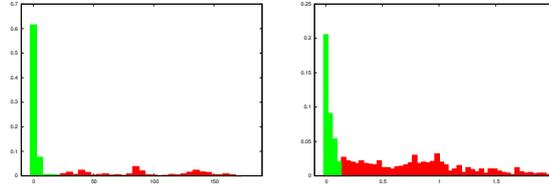
Fig. 9. Typical shape of error distributions (Gaus.Noise-160, cave,  $d = 1m$ ) with principal mode highlighted.  $|e(\phi)|$  distribution is multimodal (left),  $|e(T)|$  distribution has a peak and uniform noise (right).
