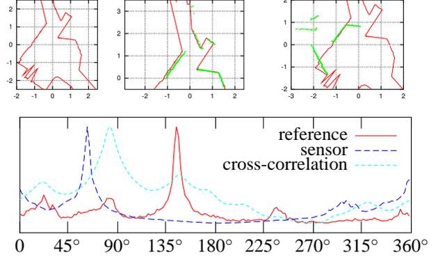
Fig. 6. In (a) it is shown the reference data, resulting from ray-tracing a map of a Nist Rescue arena. In (b) and (c) it is shown the sensor data (laser range finder, shown as points) matched according to the first two solutions given by HSM. (b) is the “exact” match, apart from map inconsistencies, however also (c) is a plausible solution.
