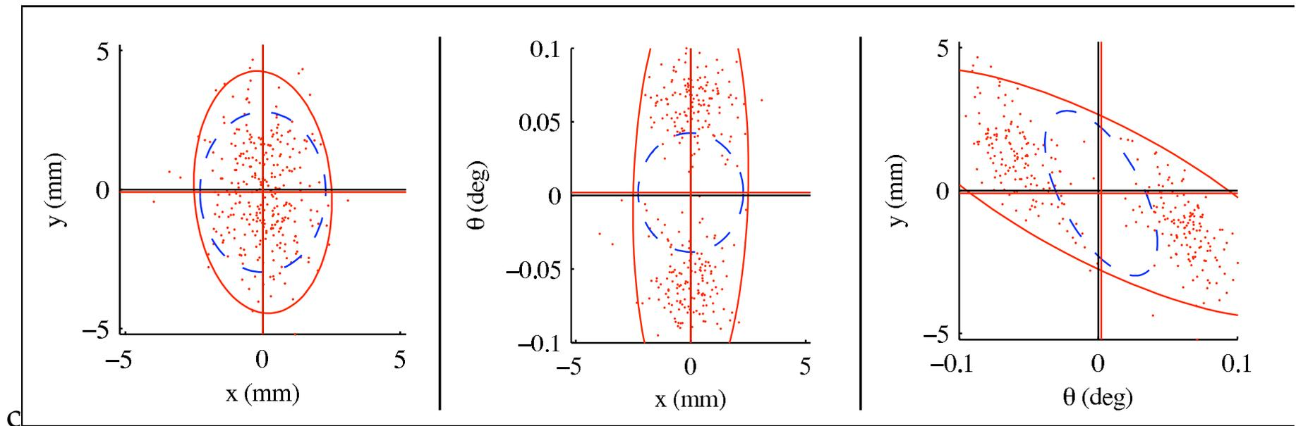
Estimation error versus error bound on the  $(x, y)$ ,  $(x, \theta)$ ,  $(y, \theta)$  planes.
