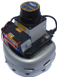
Figure 2. The Khepera III robot with an on-board Hokuyo URG-04LX range-finder used in the experiments.
